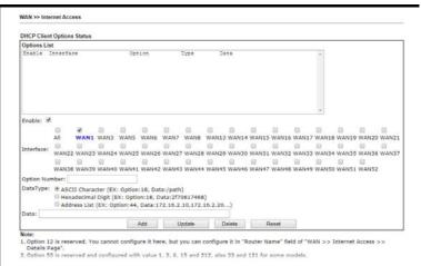
Enable - Check the box to enable the function of DHCP Option. Each DHCP option is composed by an option number with data. For example,
