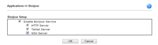
5. Open the DNSSD page again. The available items will be changed as the follows. It means the Vigor router (based on Bonjour protocol) is ready to be used as a printer server, FTP server, SSH Server, Telnet Server, and HTTP Server.
