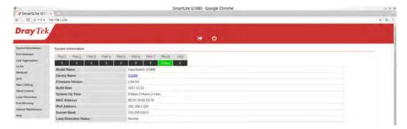
First, IP Address: as shown above, enter "192.168.1.224", for instance. For sure, an IP address such as 192.168.1.x must be set on your PC.
